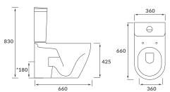
Coupling to soil stack: Straight out and straight down Distance from soil pipe
