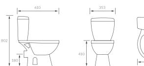
Coupling to soil stack: Straight out, straight down, Left or Right
