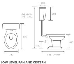
Coupling to soil stack: Straight out, straight down, Left or Right
