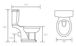
Coupling to soil stack: Straight out, straight down, Left or Right Distance from soil pipe spigot to wall: Cistern inlet position: Left
