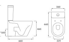
Coupling to soil stack: Straight out and straight down
